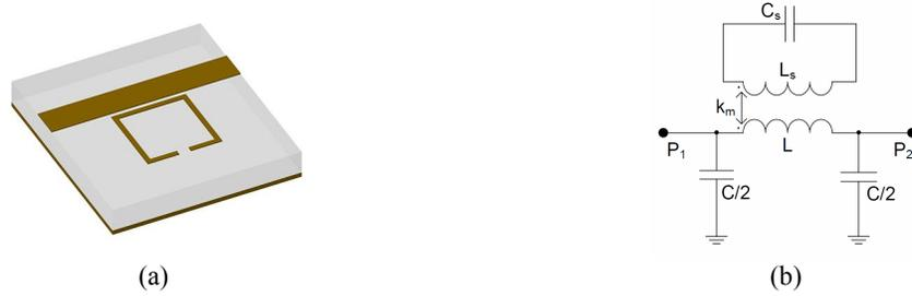
Fig. 1. (a) SRR coupled with microstrip line (b) equivalent circuit.
