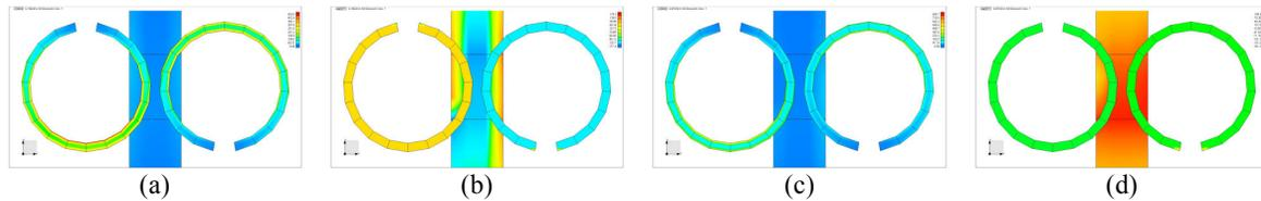
Fig. 3. Current distribution at first resonance: (a) magnitude (b) phase; at second resonance: (c) magnitude (d) phase.
