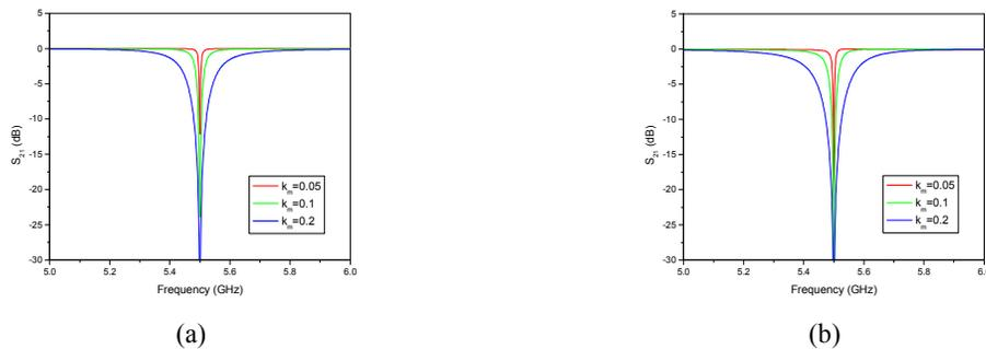
Fig. 2. Calculated logarithmic magnitude of transmission through the microstrip line coupled with single SRR using: (a) equation (2); (b) equivalent circuit in Fig. 1b.
